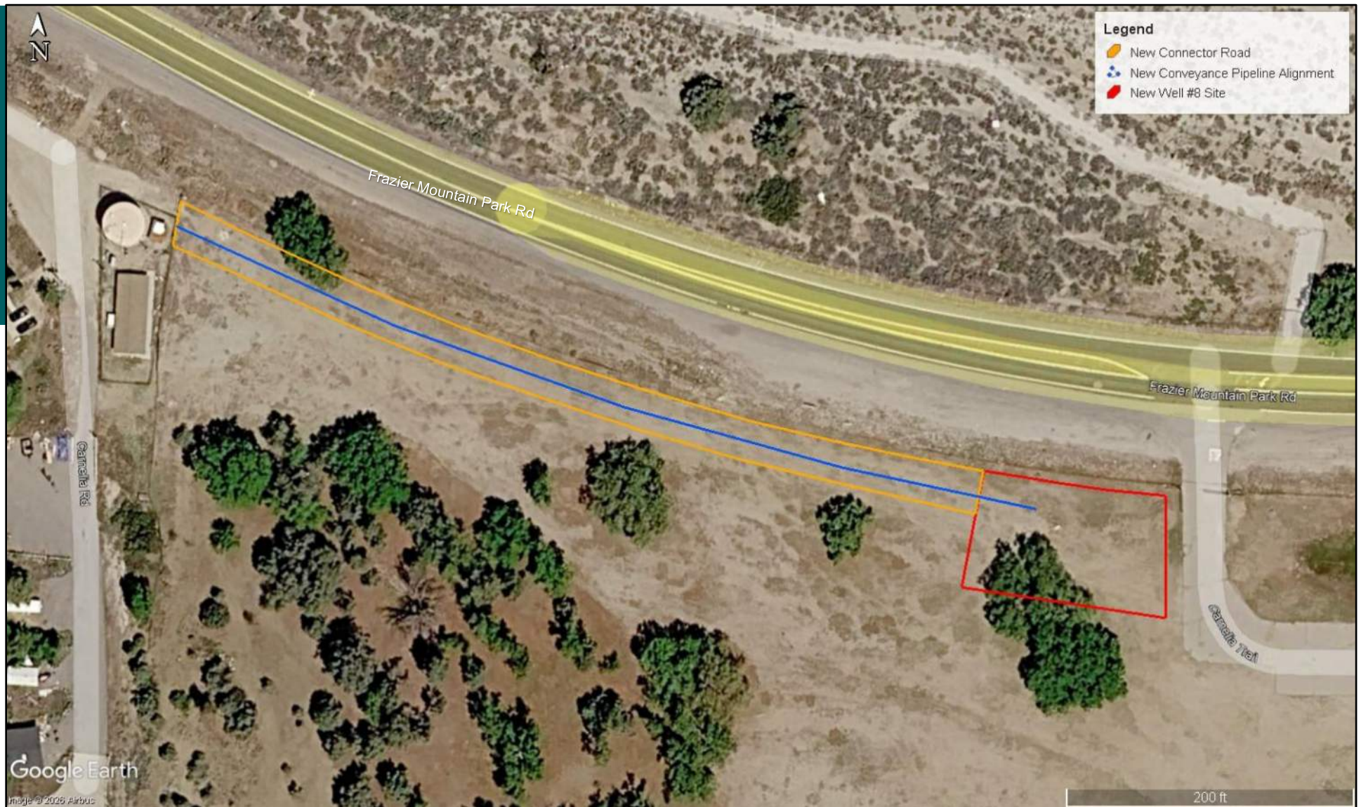
Figure 4b. Aerial Photograph of New Well #8 Site & Connector Road with Conveyance Pipeline Alignment
